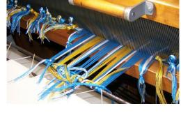
7. Sampling for tension and threading errors – It's very likely that a mistake can occur when threading and sleying over 800 threads. Checking it now for mistakes, correcting them, determining the exact right pressure to each beat to get the same number of threads in the weft per inch as in the warp takes some practice and several inches. We're ready to go ahead with the custom fabric! Total time – ½ hour.
