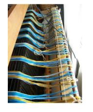
front of the loom and through the "tensioning sticks" I use to help keep even pressure on the threads, it's time to "spread" the threads through the "raddle" on the back beam. Pegs are set 1" apart, and 20 threads are placed between each one before attaching them to the warp beam in the back of the loom. Then they're tied to the "warp beam" (underneath). *Total time – 1 hour.*
